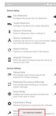
7 To enable the **iBeacon** feature which scans and returns to the online platform nearby beacons provided by IoT Solutions, ensure Vehicle Detection Mode already Enabled (Car or Trailer) and press on the switch for iBeacon Scanning.
