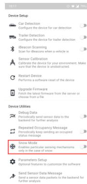
9 **Repeated Parking Occupancy** can also be enabled. In this mode, the sensor repeats the parking occupancy message after a time interval only when it becomes occupied.
