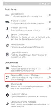
**10** The interval for the repeated parking occupancy message can be setup by pressing on the **Parameters Setup**. The interval can then be configured from the opened menu. Finally press **Send** to apply the configuration.
