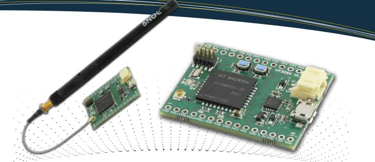
The BRKHT32SX breakout board provides an easy way to test under real operating conditions the HtMicron HT32SX Multicomponent Integrated Circuit (MCO) designed to provide a ready-to-use connectivity solution for Internet of Things (IoT) applications.
